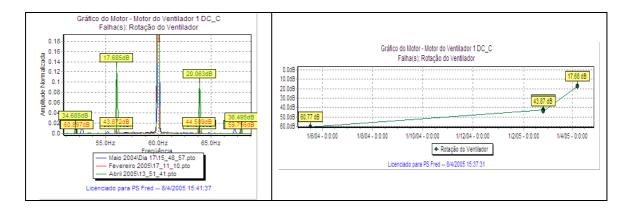
The diagnosis for this motor was: "presence of imbalance, misalignment or looseness in the fan set (including the gearbox)". The driven train was analyzed and, in fact, there was looseness in the gearbox. After repair:
